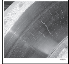
Heavy Heat Check FIGURE 107
